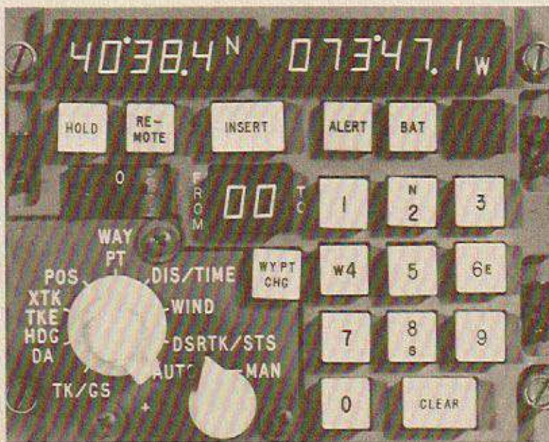
The Control/Display Unit is the pilot's communication link with the remainder of the Carousel IV system. The unit displays a wide range of navigation information.
